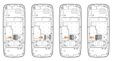
Place the microSD card with the chip facing downwards and slide it into its housing. Make sure that it is correctly inserted. To remove the card, press and slide it out.
